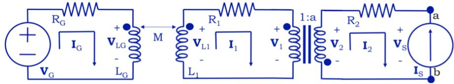
$$\mathbf{V}_G = 8 \text{ V}, \mathbf{I}_S = 1 \text{ A}, a = 2, \omega M = 0.5 \Omega,$$
