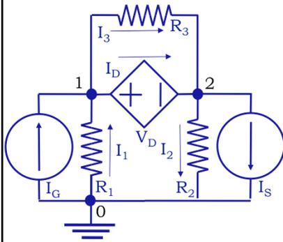
$$\begin{aligned} 1: I_G &= V_1 \left( \frac{1}{R_1} + \frac{1}{R_3} \right) - \frac{V_2}{R_3} + I_D \\ 2: -I_S &= V_2 \left( \frac{1}{R_2} + \frac{1}{R_3} \right) - \frac{V_1}{R_3} - I_D \end{aligned} \quad \left. \begin{array}{l} \text{Formulación directa} \\ \text{de las ecuaciones de nudo.} \end{array} \right\}$$
