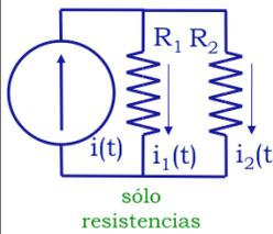
$$i_1(t) = \frac{R_2}{R_1 + R_2} i(t)$$
