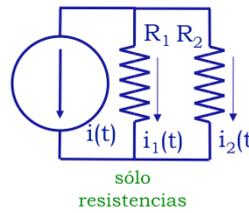
$$i_1(t) = -\frac{R_2}{R_1 + R_2} i(t)$$
