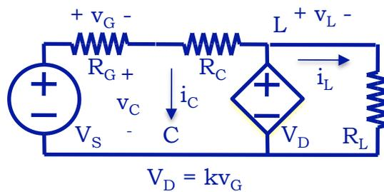
$$v_G = i_G R_G = \frac{V_S - V_D}{R_G + R_C} R_G = \frac{V_S - kv_G}{R_G + R_C} R_G = \frac{V_S - ki_G R_G}{R_G + R_C} R_G \Rightarrow$$
