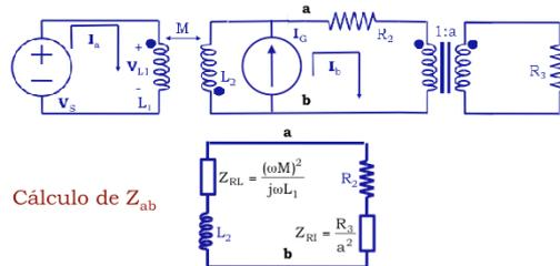
$$Z_{RL} = \frac{(j\omega M)^2}{j\omega L_1} \quad Z_{Ri} = \frac{R_3}{a^2}$$
