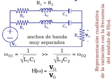
$$\omega_{01} = \frac{1}{\sqrt{L_1 C_1}} \gg \frac{1}{\sqrt{L_2 C_2}} = \omega_{02}$$
