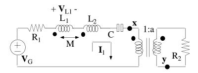
$$\begin{split} \textbf{V}_G &= 4 \text{ V}, \, \omega = 100 \text{ krad/s}, \, a = 2 \\ R_1 &= 1 \, \, \Omega, \, R_2 = 4 \, \, \Omega, \, C = 1 \, \, \mu F \\ L_1 &= 40 \, \, \mu H, \, L_2 = 40 \, \, \mu H, \, M = 10 \, \, \mu H \end{split}$$
