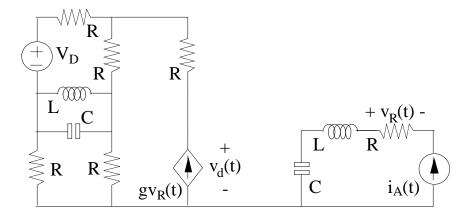
$$\begin{aligned} i_A(t) = I_A cos(\omega t), I_A = 1 \text{ A, } \omega = 1 \text{ rad/s, } V_D = 2 \text{ V} \\ R = 1 \text{ } \Omega, \text{ } g = 2 \text{ S, } L = 1 \text{ H, } C = 1 \text{ F} \end{aligned}$$
