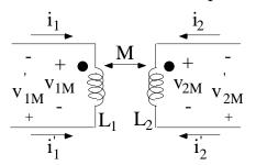
$$v_{1M} = M \frac{di_2}{dt} = -M \frac{di'_2}{dt} = -v'_{1M}$$
