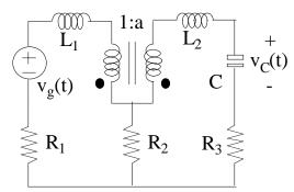
$$v_{g}(t) = V_{D} + V_{A}cos(\omega t)$$
