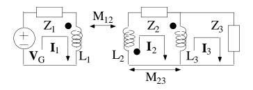
$$\begin{split} \mathbf{V}_{G} &= \text{- j54 V} \\ Z_{1} &= 2 \text{ - j4 } \Omega, \, Z_{2} = 8 \text{ - j65 } \Omega, \, Z_{3} = 23 \text{ - j36 } \Omega \\ \omega L_{1} &= 4 \, \Omega, \, \omega L_{2} = 9 \, \Omega, \, \omega L_{3} = 36 \, \Omega \\ \omega M_{12} &= 4 \, \Omega, \, \omega M_{23} = 10 \, \Omega \end{split}$$
