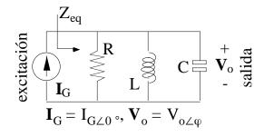
$$T(\omega) \equiv \frac{\mathbf{V}_{o}}{\mathbf{I}_{G}} = Z_{eq} = \frac{1}{\frac{1}{R} + \frac{1}{j\omega L} + j\omega C} \qquad T(\omega) \equiv \frac{\mathbf{V}_{o}}{\mathbf{V}_{G}} = \frac{R}{Z_{eq}} = \frac{R}{\frac{1}{j\omega C} + j\omega L + R}$$
